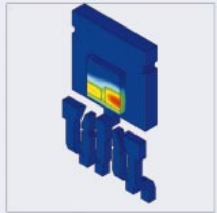
P-TO252-3-1 without mold compound with P_V = 3 \text{ W} for determining the R_{thj-c}
