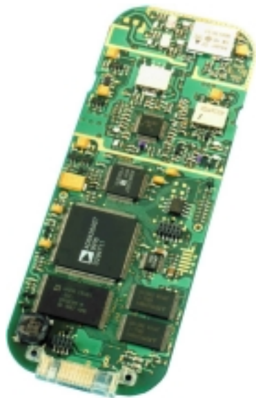
Photo 2. A six layer PCB with through and blind vias used in a GSM phone.
