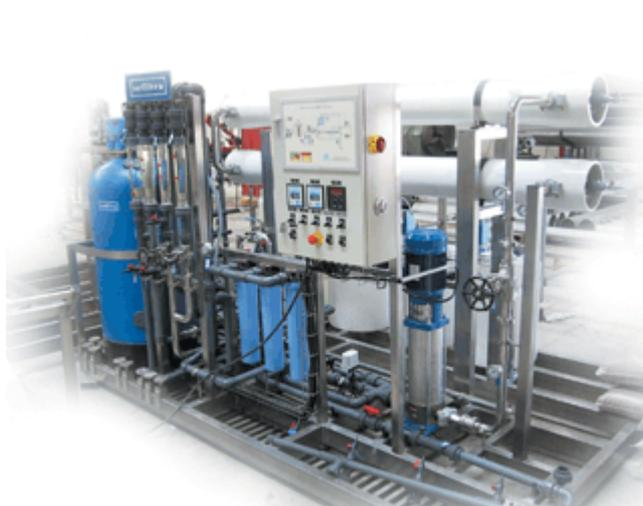
Fig. 79. A. Proceso de Osmosis Inversa<sup>12</sup>
