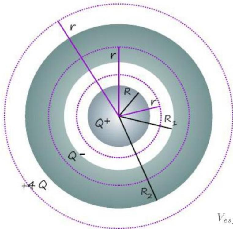
$$V_{corona} = - \int_{\infty}^{R_2} \vec{E}_{r \geq R_2} \cdot d\vec{r}$$
