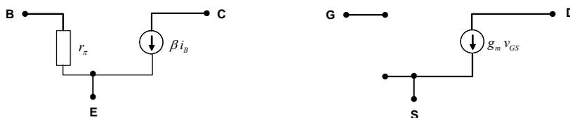
$$A_v (BJT) = \frac{V_{Out}}{V_{In}} = -\frac{\beta i_B}{r_\pi i_B} r_{POL} = \frac{\beta}{r_\pi} r_{POL} \approx \frac{200}{3000} = 0.06 \text{ (décimas)}$$
